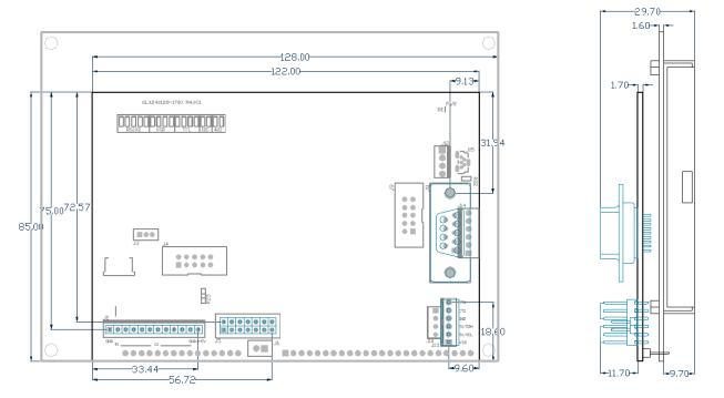
Figure 22: Standard Model Dimensional Drawing
