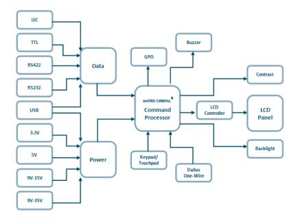
Figure 20: Functional Diagram
