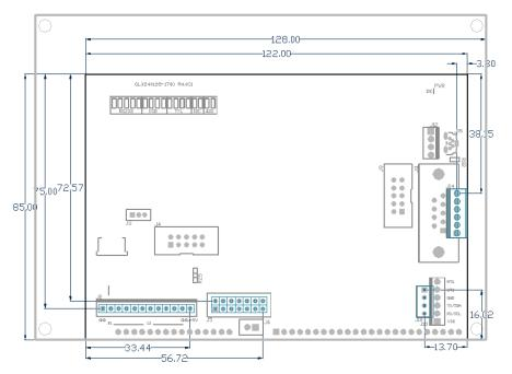
Figure 24: RS422 Model Dimensional Drawing
