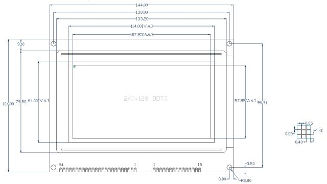
Figure 21: Display Dimensional Drawing
