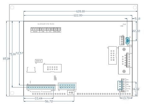
Figure 23: USB Model Dimensional Drawing
