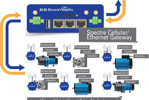
Wzzard™ Intelligent Edge Nodes/ Wireless SmartMesh IP Sensor Network
