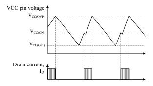
Figure 10-12 OVP operational waveforms
