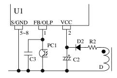
Figure 10-10 FB/OLP pin peripheral circuit
