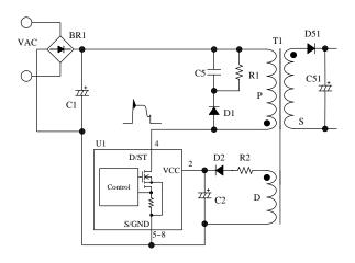
Figure 11-3 D/ST pin peripheral circuit
