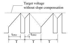
Figure 10-7 Drain current, I<sub>D</sub>, waveform in subharmonic oscillation
