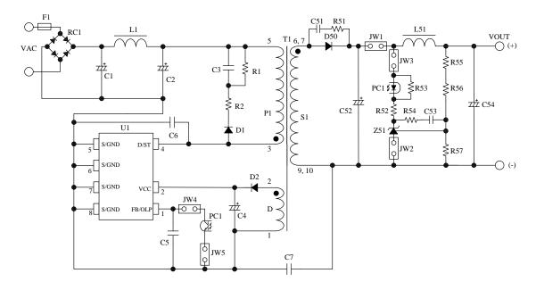
Figure 12-2 Circuit schematic for PCB circuit trace layout
