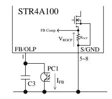
Figure 10-5 FB/OLP pin peripheral circuit
