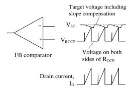
Figure 10-6 Drain current, I<sub>D</sub>, and FB comparator operation in steady operation
