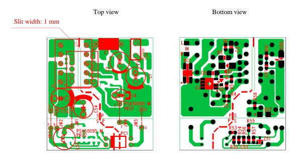
Figure 12-1 PCB circuit trace layout example (SOIC8 type)
