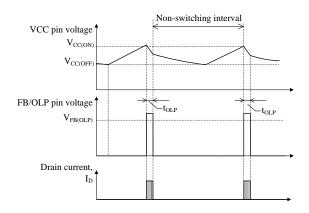
Figure 10-11 OLP operational waveforms
