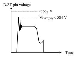
Figure 11-4 D/ST pin voltage waveform in normal operation
