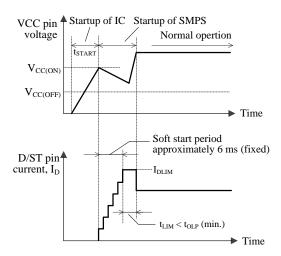
Figure 10-4 V<sub>CC</sub> and I<sub>D</sub> behavior during startup
