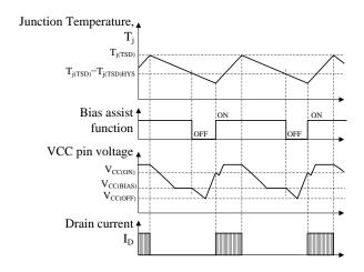
Figure 10-14 TSD operational waveforms
