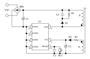
Figure 11-1 The IC peripheral circuit
