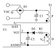
Figure 10-1 VCC pin peripheral circuit
