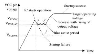
Figure 10-3 VCC pin voltage during startup period
