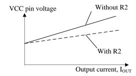
Figure 11-2 Variation of VCC pin voltage and power
