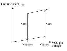
Figure 10-2 Relationship between VCC pin voltage and I<sub>CC</sub>
